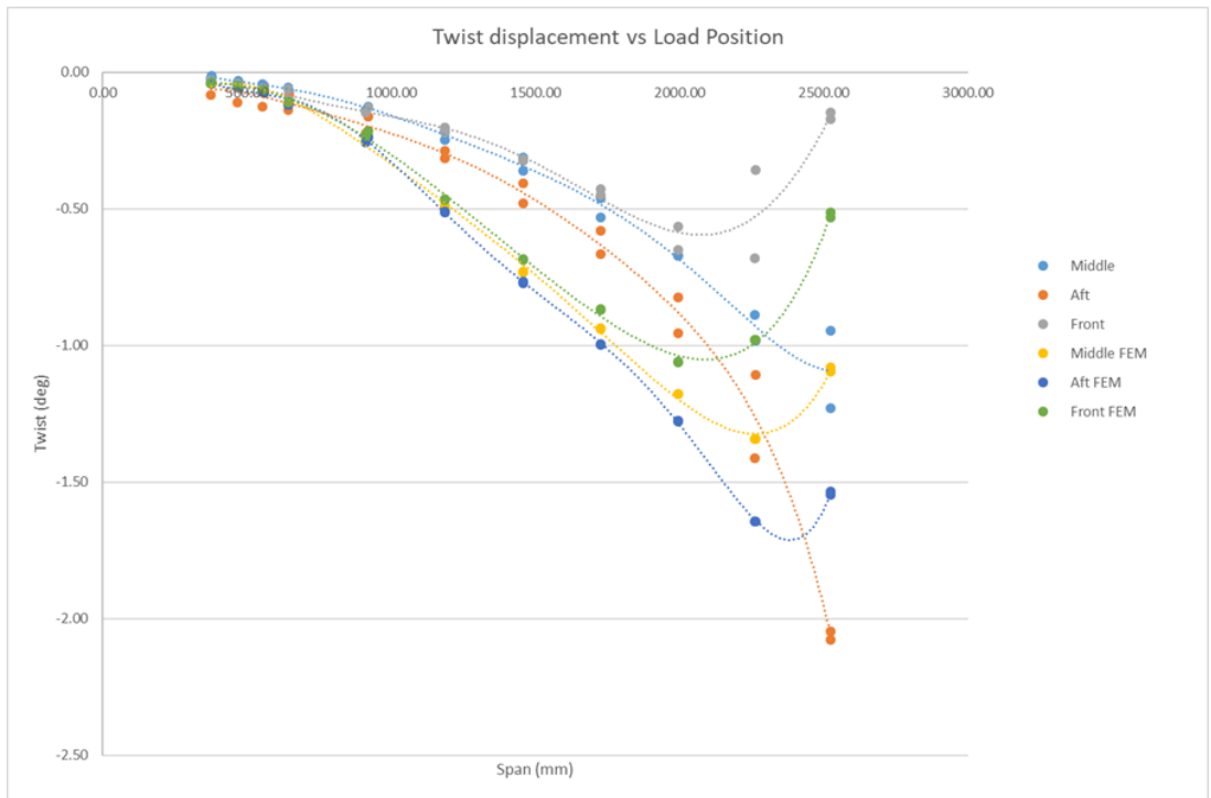
Figure 4.10: Comparison between experimental and FEM twist displacement results for different load positions (cases 3, 4 and 5).
