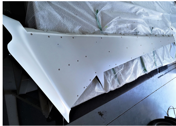
(b) Fiducial stickers placement on the wing
