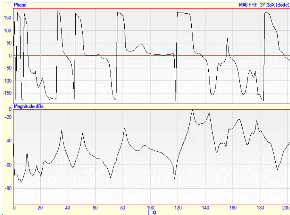
(b) Post processed FRF measured in X direction.
