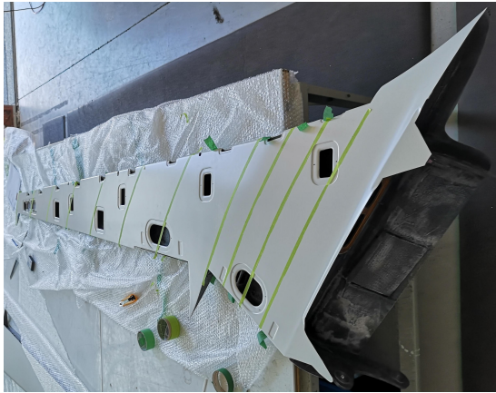
(a) Tape lines to help finding the exact position of fiducial stickers.
